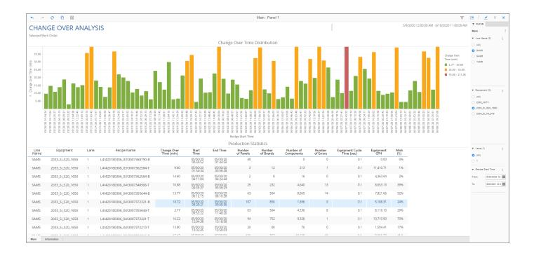
This report displays detailed changeover information for each line, piece of equipment and lane in the factory. It shows the changeover time distribution and overall production statistics per work order, including number of boards, number of errors, cycle time, components per hour (CPH) and work percentage.
